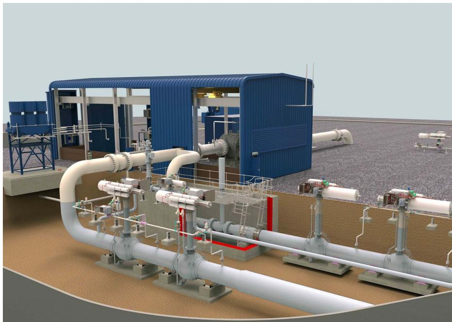
Example of a 3D model of an Above Ground Installation.
