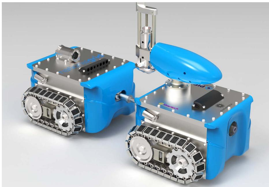
The twin chassis design of the robot.
