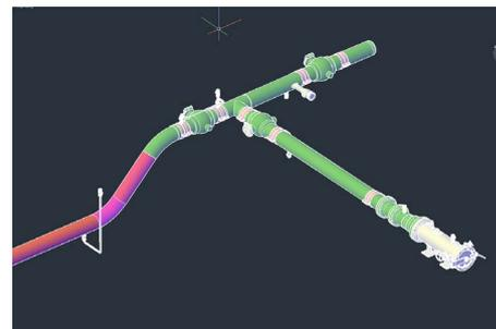
Figure 7 – Pannal AGI pipework with PIE GRAID model condition colour-coding example.
