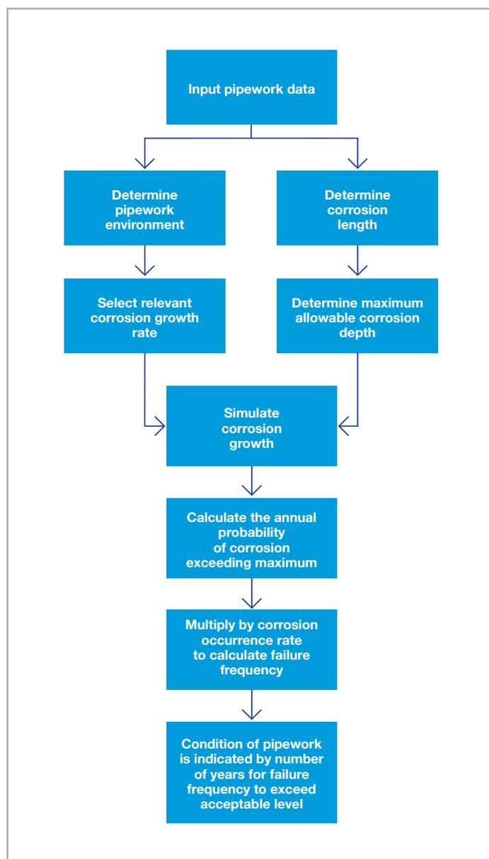
Figure 6 – Probabilistic corrosion growth model for calculating pipeline inspection interval.
