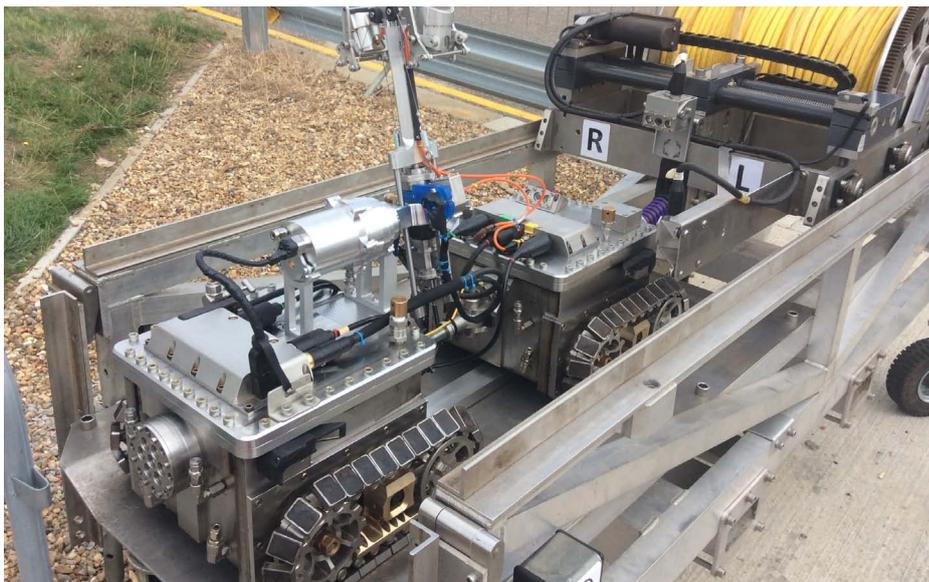
The robotic platform including robot, UMS, tether and transportation trolley.
