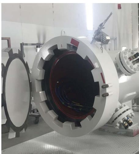
The launch vessel quick closure door (above) and the final test loop (right).
