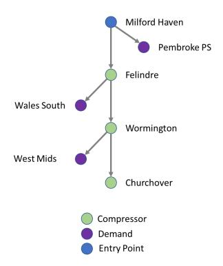
Figure 1: Schematic representation of the key NTS assets that have an influence on Milford Haven Entry capability
