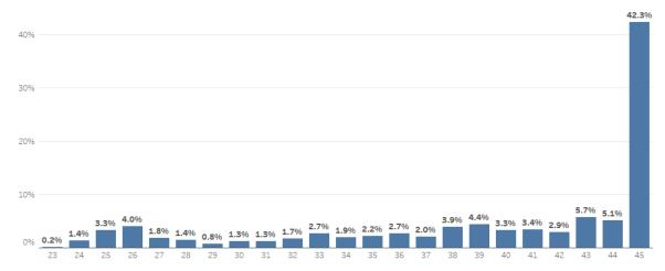
Figure 2: Overview of recent flow rates through Churchover Compressor. The figure identifies 45 mcm/d as the maximum achievable flow. N.b. Churchover Unit D used as the alternative unit will be on outage over the summer period
