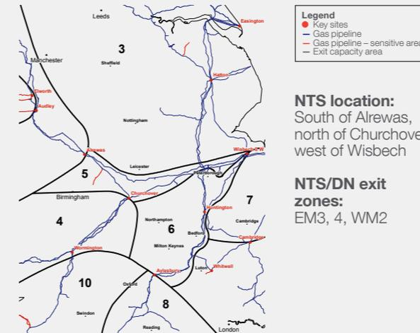
The unsold capacity here indicates a limited scope for substitution. Potential non-Planning Act reinforcements could be carried out to release a small amount of capacity, but significant pipeline reinforcement would be required, particularly for the sensitive area on Feeder 14 between Austrey to Shustoke.
