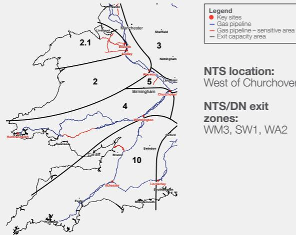
Exit capacity availability is highly sensitive to Milford Haven flows. Low Milford Haven flows result in reduced South Wales pressures, which limit capacity. High Milford Haven flows result in reduced pressures in the West Midlands which may limit capacity.
