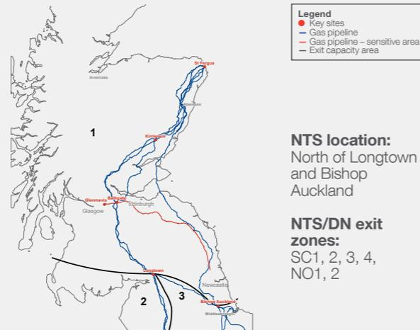
This region is sensitive to St Fergus flows. High St Fergus flows mean that exit capacity will be available, as flows from the St Fergus terminal are predominately in a north to south direction. As St Fergus flows reduce, exit capacity will be constrained.
