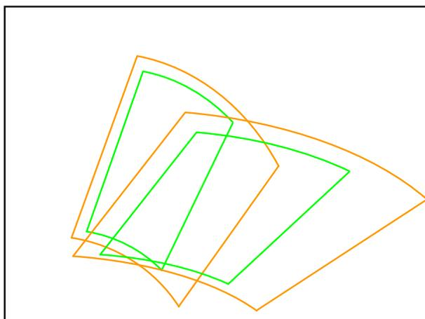
Figure 3 – Use of dissimilar overlapping compressors to increase range of high efficiency operation
