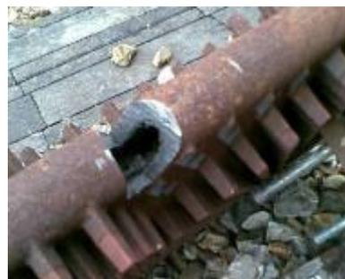
(NB: The iron fillings present are from the cutter not internal corrosion.)
