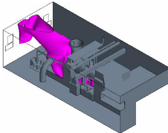
CFD prediction of gas accumulation in a compressor cab
