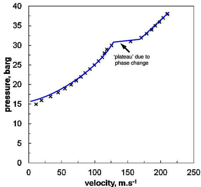
Figure 6 Typical decompression vs velocity plot
