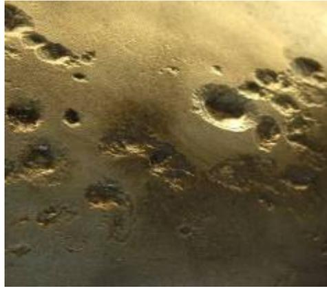
Figure 3: Area of corrosion pitting found on Partington pipe.
